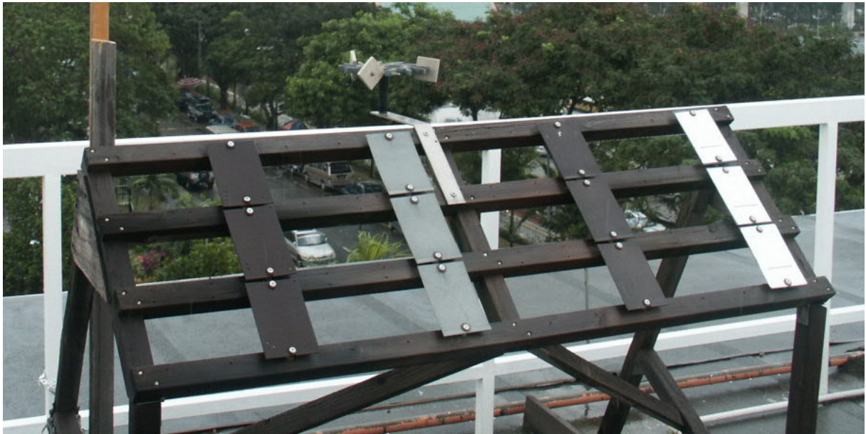
Fig. 8. Metal plates mounted on a typical exposure rack made of wood, facing south at the northern hemisphere, or north at the southern hemisphere, at an angle of 45^\circ to the horizontal. The plates are fastened to the rack with stainless steel screws using plastic insulators.
